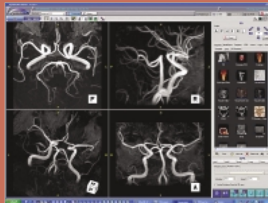
By using the AquariusNET server, the MIP processing can be performed on-the-fly in real time, providing the radiologist with complete control and removing the need for time-consuming additional processing at the scanner by the technologist.
