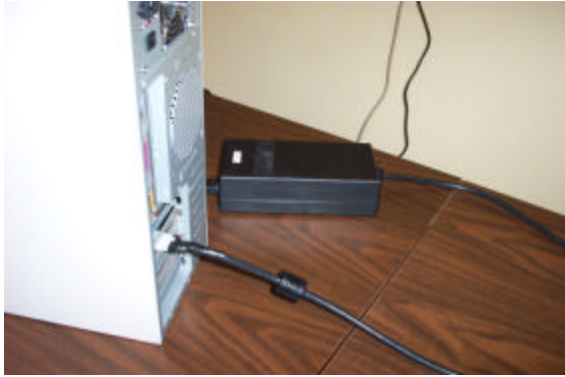
Examples of proper VolumePro 1000 External Power Supply Cables installation
