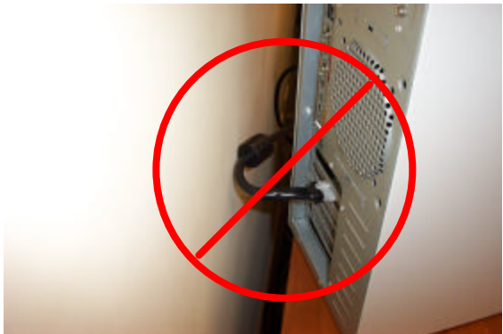
Examples of improper VolumePro 1000 External Power Supply Cables installation
