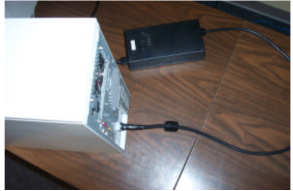
Examples of proper VolumePro 1000 External Power Supply Cables installation
